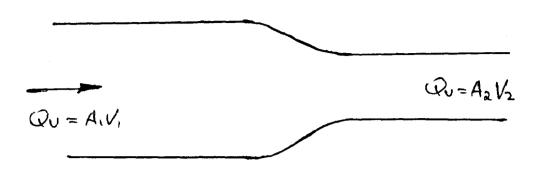
Force on nozzle =  $\ell \times Q_V \times (V_2 - V_1)$
