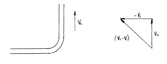
The change in velocity =  $V_2-V_1$ .  $(V_2-V_1)$  is the direction in which the force has to be applied to prevent the pipework moving.
